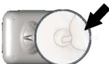
Remove the protective film from the suction cup.
