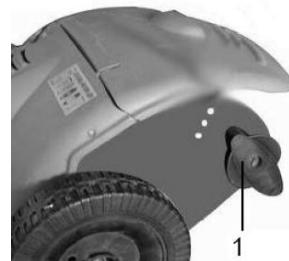
The working depth is adjustable to 3 heights. Pull adjustment arm (1) away from side cover and allow catch in desired position (2). Adjust the height alternately left and right by only 1 position. The adjustment arms must always be in the same height position.
