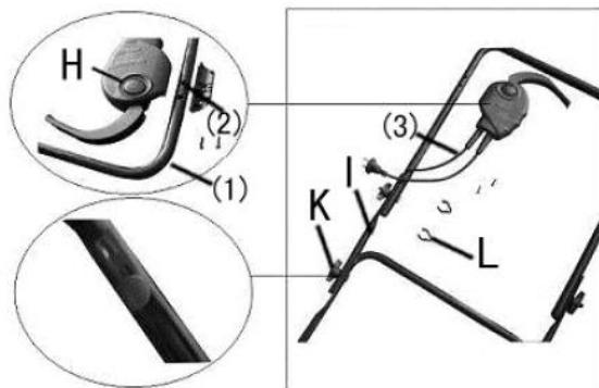
Fasten switch cable with the clips (L) on the handle rod.
