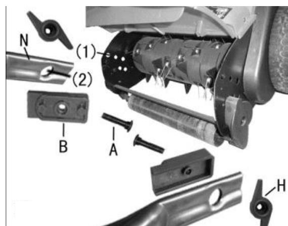
Insert securing screw (A) form inside through the left side element. Position insulation element (B) from outside; the two nubs must catch in the holes of the side element (2). Place insulating element (B) so that the large opening points to the outside. Position tip of handle element (N) in the insulating element (B). Then tighten wing nut (H).
