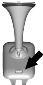
Press the button at the middle bottom of the back to release the device.
