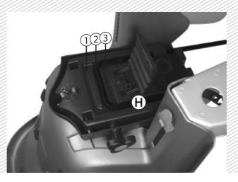
In order to adjust the baby seat onto the bicycle, put the metallic rod into one of the three allowed positions.
