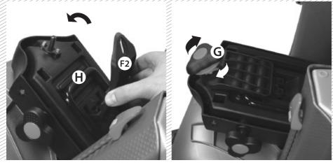
Close the plastic mounting plate (F2); make sure it holds the metallic bracket (H) and fasten the hand knob (G).
