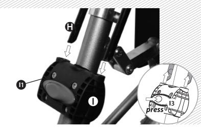
Insert the ends of the metallic bracket (H) into the holes of the mounting block (I) until you hear a click that signals it is in the locked position. Centre and adjust the seat above the rear wheel. Make sure the seat does not touch the rear wheel when you add the child's weight. Tighten the screws (I1) securely. Try to shake the seat to make sure it is secure on the bicycle. To remove the seat, press the block button (I3) and remove it according to the direction indicated in the picture.
