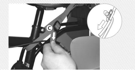
Pass the safety belt (C) around the bicycle frame. Adjust it as shown in the picture, under tension.
