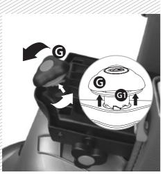
Unscrew the hand knob (G) and simultaneously lift the red security ring (G1).
