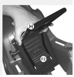
Hold the metallic bracket (H) the same as in the picture and pass it through the opening in the baby seat.
