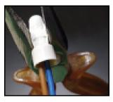
Note: Do not cut the old crimp as this causes shortening of the wires and can be an issue afterwards. Always connect the wires with a new 2 or 3-wire crimp housing.
