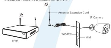
Notes: When WIFI signal is not strong enough against walls, users can take off the original antenna and subtitute antenna extension cord. Drill a hole on the wall to let the extension cord go through and simply put it where WIFI signal is strong. Note: The extension is not part of the package
