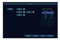
Step 3. As picture shown below, it means IPC1 is connected to NVR through IPC2 and IPC3. IPC2 is connected to NVR through IPC3. IPC3 is connected to NVR directly.
