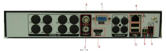
(1) Audio output (2) HDMI (3) USB (4) RS485 (5) Power (6) BNC (7) VGA (8) Network The rear panel of enhanced equipment
