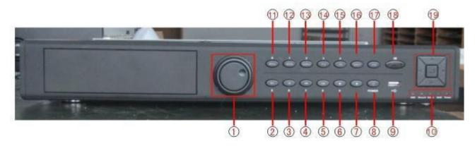
(1) Shuttle (2) Play Pause (3) Slow Play (4) Fast Play (5) Backwards Pause (6) Play back Stop (7) Record (8) Power switch (9) USB mouse (10) Indicator light (11) Main menu (12) Scene switch (13) Record check (14) PTZ (15) Assist (16) Shift (17) ESC (18) IR remote receiver (19) Direction
