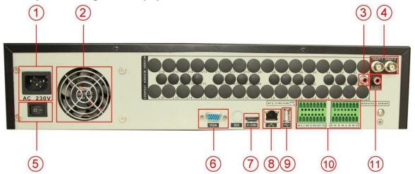
(1) Power (2) Cooling mouth (3) Audio Input (4) Video output (5) Power switch (6) VGA Interface (7) HDMI (8) Network (9) USB (10) External (11) Audio output
